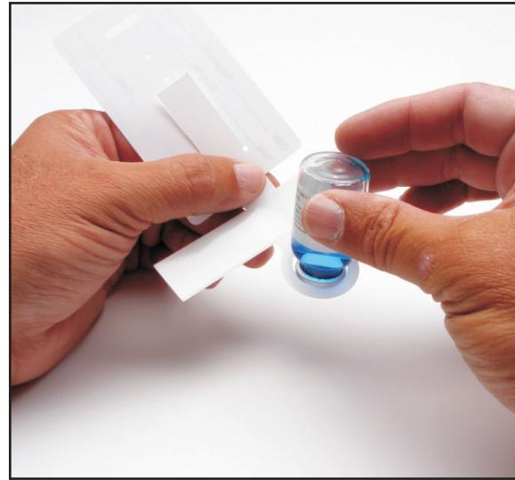
5) Pull down the central tab on the vial holder. Fold it across the bottom of the vial and then along the side.
