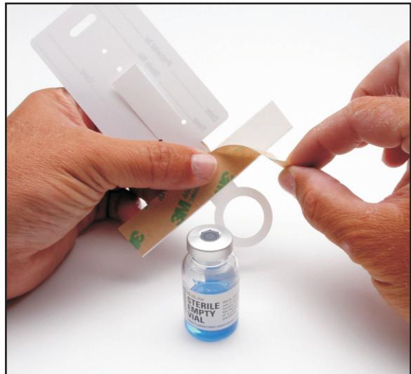
4) Slip the loop of the vial holder over the neck of the serum vial, as shown:
