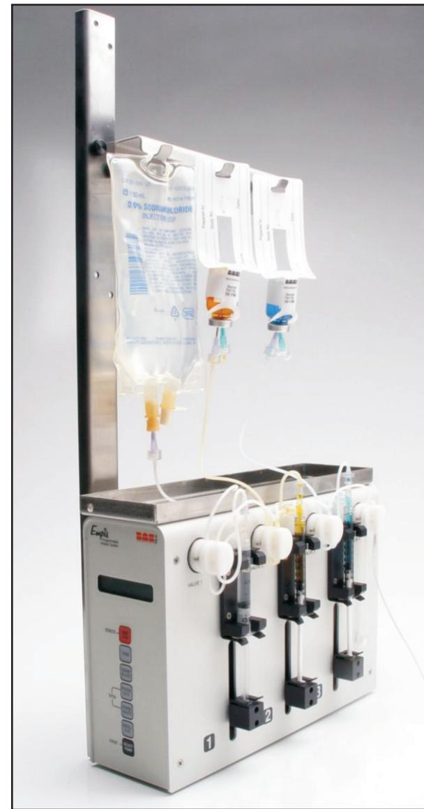
11) Hang the vial of solution on the Empis rack, as shown, and complete the connection to refill line on the appropriate syringe.
