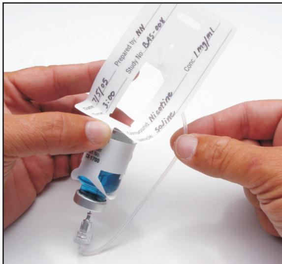
10) Thread the vent tube in and out of the two small holes at the top of vial holder to keep it secure and upright.
