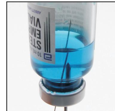
12) Ensure that the refill needle will remain below the surface of the solution in the vial. If there is too much tension on the refill line, lower the height of the rack or adjust the refill line as needed.
